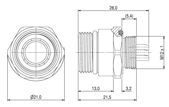
Note: Mounting hole must have M12 x 1 thread
