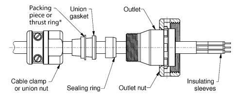
Solder conductors to connector contacts.
