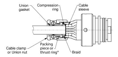
\* - Metal thrust ring is supplied with LMA/1/81087/203 and LMA/1/81089/203 accessory sets.
