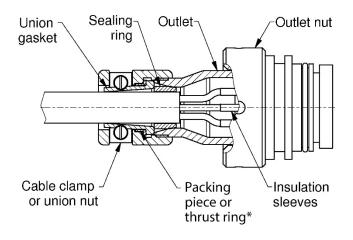
\* - Metal thrust ring is supplied with LMA/1/81087/203 and LMA/1/81089/203 accessory sets.
