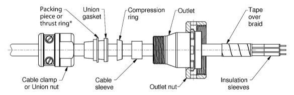
Solder conductors to connector contacts and slide insulating sleeves over soldered joints.
